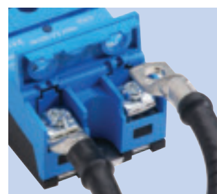
With tips with contained palm Up to 25mm 2 (AWG4) i.e. 85A Up to 50mm 2 (AWG1) with or without special adaptations i.e. 150A
