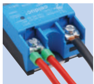
Direct connection by wire or tip 2 x 6 mm 2 (AWG10) fine strand i.e. 32A 2 x 10 mm 2 (AWG8) solid i.e. 50A
